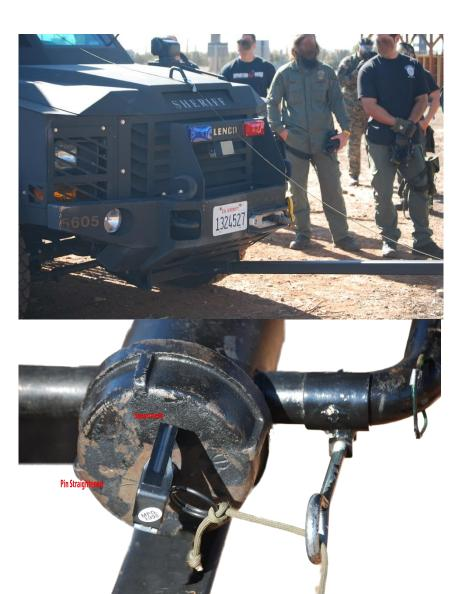
Close up of grenade cord attachment. Note that grenade safety pin is straightened for easier remote removal
